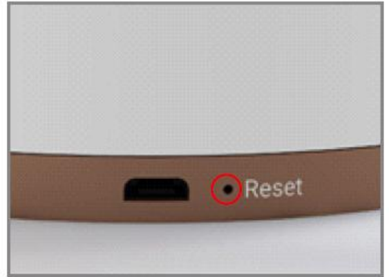
PT camera Reset button is at the bottom of the camera (next to adapter input)
