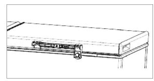
1. Fix the handle on the door with screws.
